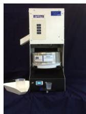
Sievematic Grain Shaker and Sievematic II Auto Test Weight and Screenings System
