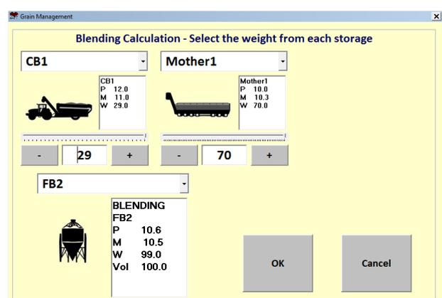
Once the operator presses the OK button, the data is sent to the CropNet internet web site. From the CropNet web site, the farmer or anyone he provides access, can view the data using a Smart Phone, Tablet or PC. The data can then be downloaded to a PC running the CropNet Grain Data Management Software.
