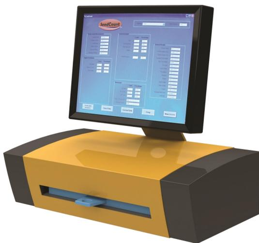
Seeds are spread over the sample tray and inserted into the SeedCount scanner module. The SeedCount software draws a border around each seed and uses the pixels within the border to define each parameter.
