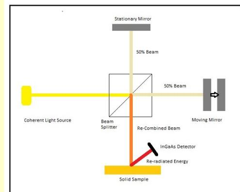
interference. The detector scans the re-combined beam over the time it takes for the mirrors to move in and out of phase. The signal collected by the detector is the interference pattern but it is called an Interferogram.
