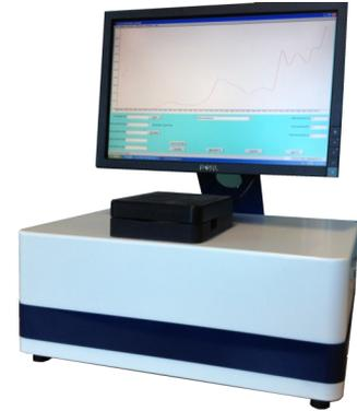
The Series 4000 is based on a Michelson interferometer using a InGaAs detector. The systems offers far superior performance over dispersive NIR spectrometers.
