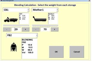
content of 10% is placed into Field Bin2 would produce 99 tonne of wheat with an average protein content of 10.6%. In effect the ASW wheat from the Mother Bin was blended up to APW using grain from Chaser Bin1. The Blending Calculator is intended to take the guesswork out of in field blending.
