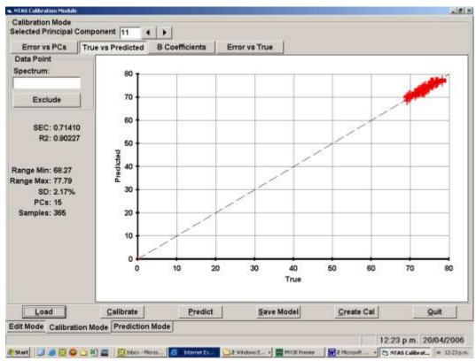
Figure 1: Moisture Calibration plot
