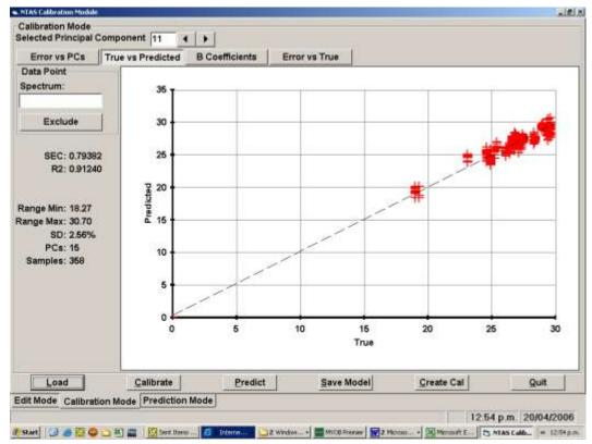
Figure 4: Calibration plot for Brix
