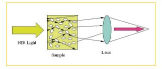
Within this region of the electromagnetic spectrum, N-H (protein), C-H (fats and oils) and O-H (water) and C-O-H (carbohydrates) absorb NIR light at specific frequencies. The NIT spectrum contains information about the concentration of these components. Calibration models, stored in the CropScan's computer, converts this information to % Protein, % Moisture, % Oil and % Starch and displays the results on the screen.
